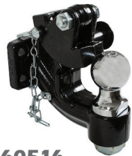
160516 ■ 2" ball ■ Forged steel w/ forged steel ball ■ Draw bar eye inner dia.: 2.38" - 3.00" ■ 10-ton capacity
