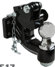
160517 ■ 2.3125" (2 5/16") ball ■ Forged steel w/ forged steel ball ■ Draw bar eye inner dia.: 2.38" - 3.00" ■ 10-ton capacity
