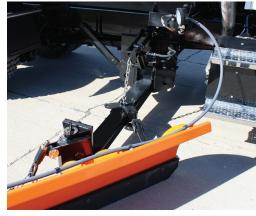
Extension cylinder mounted inside the cross tube for protection from road debris. Lift arm design eliminates slide construction which can bind.
