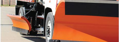
Unit tucks straight back for minimal interference, leaves room on body for ladders, shovel holders, tarp hooks, etc.
