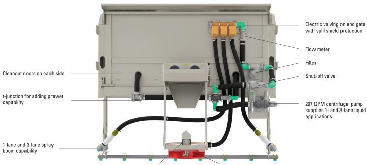
Hydraulic motor 2.8 CIR for spinner 18" poly spinner
