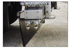
OPTIONAL: Air flow baffle mounted ahead of the liquid spray boom helps prevent drift due to travel speed and wind turbulence.
