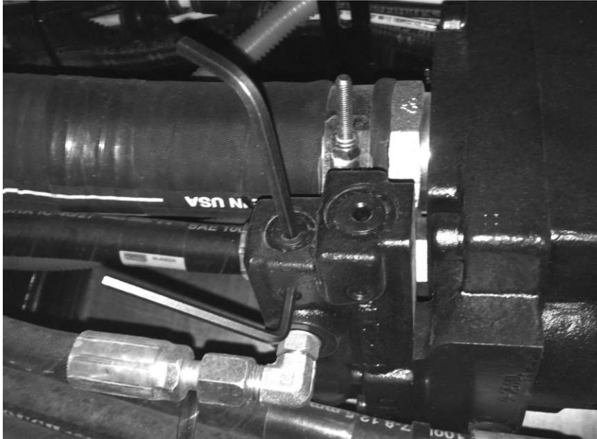
3. Set pump Stand By pressure to a minimum setting of 550 PSI as seen on gauge.
