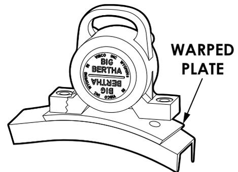
**Note:** A loose vibrator can cause damage to the bin and may also get electrically overloaded, which could cause motor burnout. Be sure to install a safety chain or cable to vibrator. Adhere to any other local, state or federal safety codes that may apply.
