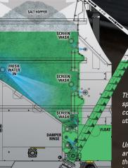
The cross-flow spray bars ensure complete salt utilization.
