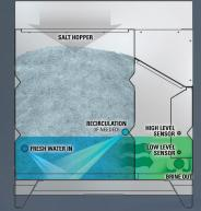
Undissolved solids are removed through the large opening. Cross-flow brine transfer for splashfree performance.
